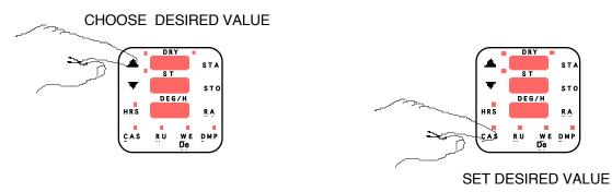
To prevent circuit over loads when starting several kilns on the same power line after a power failure a time delay can be programmed to stagger the starts of individual kilns.
