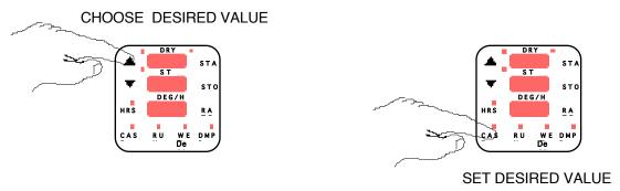
If several DCS-3000's are connected to a computer you will need to uniquely identify each DCS-3000. In SETUP mode a 3 digit identification number can be assigned to each DCS-3000. The top display will read 1d, meaning identification. Choose the desired value with the arrow keys. Press the lower left unmarked key to set this value.
