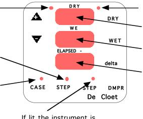
If lit the instrument is controlling STEP2 of a cure cycle.
