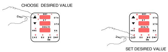
The top display shows "Str" and the middle display flashes a number from 32 to 112. Choose the desired value with the arrow keys. Press the lower left unmarked key to set this value. The operating range will always be 100 Fahrenheit degrees. It will normally be from 70 to 170. Optionally it may be changed to say 35 to 135 for Ginseng drying or 100 to 200 for drying peppers.
