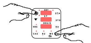
If the actual wet bulb temperature is below the set point the damper will remain closed. As soon as the wet bulb temperature exceeds the set point the damper will begin to open gradually until it is fully open when the actual temperature reaches the set point plus 2 1/2 degrees.
