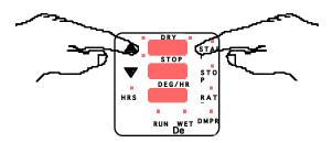
Software identification: After 10 seconds has elapsed and as long as you continue to hold the two keys the top display will read 98 and the middle display will read r0x. This indicates the version of the software which is installed. This information is helpful to our technicians.
